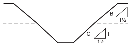
FIGURE B.1.4.1(f) B over C. [Source: 29 CFR 1926, Subpart P, Appendix B, Figure B-1.4.1(f)]
