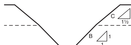
FIGURE B.1.4.1(c) C over B. [Source: 29 CFR 1926, Subpart P, Appendix B, Figure B-1.4.1(c)]
