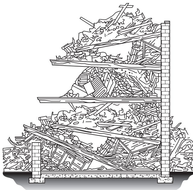
FIGURE A.5.2.2(6)(d) Cantilever Floor Collapse. (Courtesy of U.S. Department of Civil Defense)
