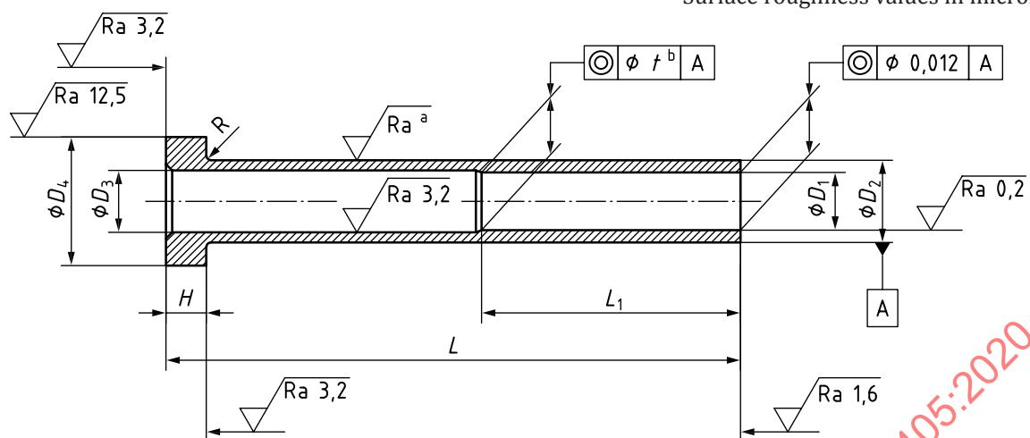
a Ra 0,8 for hot worked steel. Ra 0,4 for alloyed cold worked steel.
